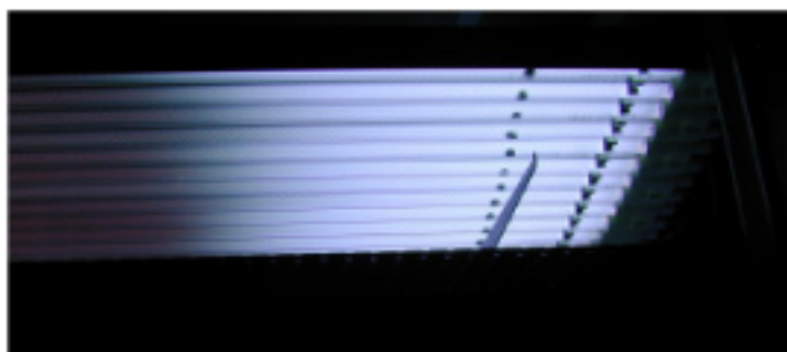
Lightpanel with 7 bulbs in U-shape-form Treatment are of 100 x 40 cm
